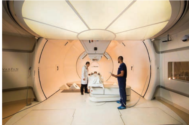
California Protons offers three gantry-style treatment rooms, allowing the proton beam to be rotated 360 degrees around the patient for greater accuracy.
